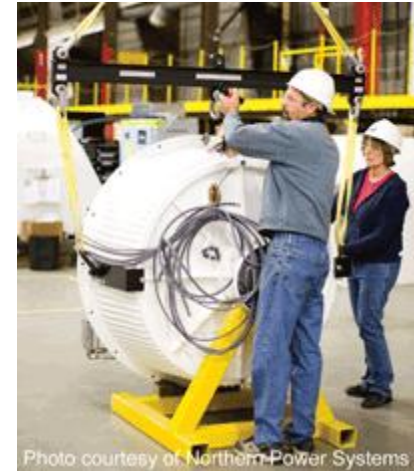
Photo courtesy of Northern Power Systems A finished wind generator is placed on a crane by turbine manufacturer North Power Systems. The company has begun adopting quality and supplier integration systems from other industries.
