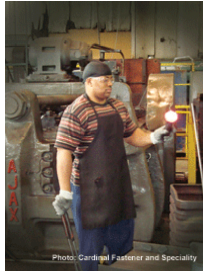
An operator at Cardinal Fastener & Speciality heat treats a fastener, which will be used to hold together wind tower segments.
